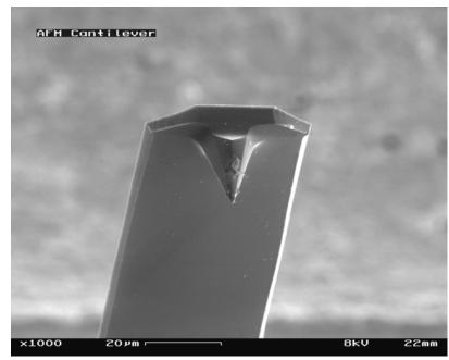
• Typically, the deflection is measured using a laser spot reflected from the top of the cantilever into an array of photodiodes. Using a Wheatstone bridge, strain in the AFM cantilever due to deflection can be measured.
